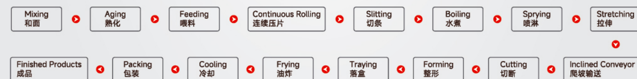
Flow Chart of Pre Cooked Fried Yee Mee (Crispy Noodles) Production Line 预煮油炸伊面工艺流程
